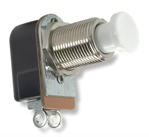
The P27-Series pushbutton switches are single pole, AC rated switches suitable for general purpose applications with a shallow back panel. These switches are momentary action with a medium actuation force (26 oz. typical). The P27-Series switch is equipped with a slow-make, slow-break contact mechanism, rated at 6 amps with a nylon concave pushbutton.
