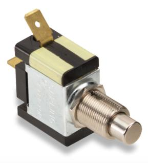
These rugged pushbutton-type switches feature international approvals, ratings to 20A 125VAC and a heavy actuation force (3-5 lbs. typical) which makes this switch ideal for use as a "foot-pedal" switch. The metal bushing and plunger construction enables this alternate action switch to withstand the rigors of most any stringent pushbutton application.
