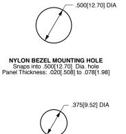
THREADED BUSHING MOUNTING HOLE Fits into .375[9.52] Dia. hole Bushing Length: .312[7.92]
