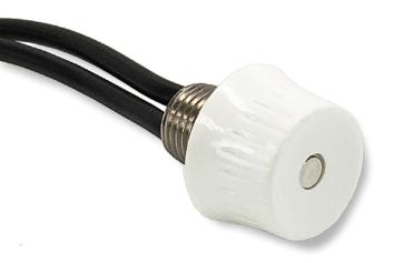
The R135 and R135A-Series rotary switches are single pole, single throw "L" rated up to 3A, feature an ON-OFF repeating action, and are available with a nylon actuating knob; nylon snap-in bracket or nickel-plated brass bushing. These switches are typically used to control lighting functions.
