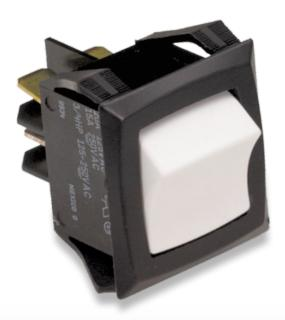
The double pole version of the R-Series incorporates the same sleek lines as the original Curvette, in a double pole envelope. Features include silver-plated butt-action contacts which afford ratings to 20A/125, 15A 250VAC and withstand peak inrush currents up to 100 amps. Paddle or rocker actuators and a choice of solder lug, .250 Tab and wire lead terminations enable this switch to adapt to high current applications.
