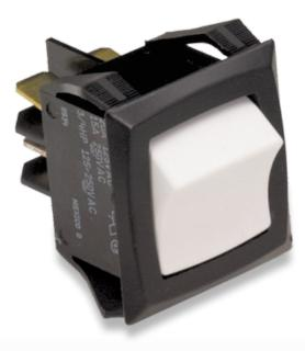
The double pole version of the R-Series incorporates the same sleek lines as the original Curvette, in a double pole envelope. Features include silver-plated butt-action contacts which afford ratings to 20A/125, 15A 250VAC and withstand peak inrush currents up to 100 amps. Paddle or rocker actuators and a choice of solder lug, .250 Tab and wire lead terminations enable this switch to adapt to high current applications.
