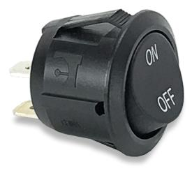
The RR and LRR-Series round rocker switches feature a uniquely sculpted rocker design with electrical ratings of up to 12A 125VAC, 10A 250VAC and fit an industry standard cutout, making installation a snap. The lighted LRR-Series can be wired to accommodate dependent or independent, illumination, neon or incandescent lamps with red, green, amber or white translucent rockers. Standard or custom actuator legends are available.
