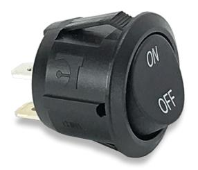
The RR and LRR-Series round rocker switches feature a uniquely sculpted rocker design with electrical ratings of up to 12A 125VAC, 10A 250VAC and fit an industry standard cutout, making installation a snap. The lighted LRR-Series can be wired to accommodate dependent or independent, illumination, neon or incandescent lamps with red, green, amber or white translucent rockers. Standard or custom actuator legends are available.
