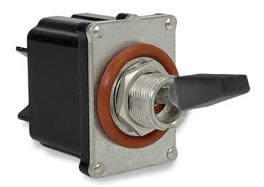
Designed to conform to MIL-DTL-3950G requirements for environmentally sealed toggle switches, and compliant to UL 60079-15 standard for use in explosive gas atmospheres. The ST-Series is fully sealed to IP68, including below the panel and features innovative design and performance principles sure to withstand the most demanding applications.
