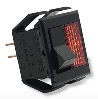
The TLG-Series Mid-Sized Tippette snap-in rocker switches are single pole, rocker or paddle actuated with an adjacent indicator light. These single-actuatorswitches are AC rated to 15 amps and are also suitable for low voltage DC applications.
