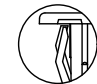
DETAIL VIEW VHP, VHP3 & VHP5 HOLE PLUGS (No wing serrations for ease of removal)
