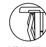
DETAIL VIEW VH1, VH3 & VH5 HOLE PLUGS (No wing serrations for ease of removal)
