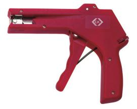
Features & Benefits  $\sim$  Designed for automatic tensioning and trimming of cable ties  $\sim$  Glass fibre reinforced polyamide construction  $\sim$  light and strong  $\sim$  Tension adjuster for the perfect tensioning of different widths of cable ties  $\sim$  For cable ties from 2,4  $\sim$  4,8 mm
