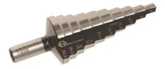
Features & Benefits ~ Centres, drills and deburs sheet metals in one operation ~ HSS, precision ground for accurate drilling ~ Dual flute construction for faster drilling & longer life ~ Three flats on drive shaft for secure drive in drill chucks ~ Cuts hole sizes: 6, 9, 12.5, 15.2, 18.6, 20.4, 22.5, 25.5, 28.3 & 30.5mm (PG7, PG9, PG11, PG13, PG16, M25, PG21),
