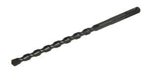
$\sim$  Tungsten carbide tipped with optimized geometry for drilling concrete and stone  $\sim$  Vacuum brazed tips for durability  $\sim$  Ground flutes designed for optimum debris removal  $\sim$  SDS-plus shank  $\sim$  Diameter: 18 mm  $\sim$  Working length: 350 mm  $\sim$  Total length: 450 mm Features & Benefits
