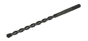
$\sim$  Tungsten carbide tipped with optimized geometry for drilling concrete and stone  $\sim$  Vacuum brazed tips for durability  $\sim$  Ground flutes designed for optimum debris removal  $\sim$  SDS-plus shank  $\sim$  Diameter: 20 mm  $\sim$  Working length: 950 mm  $\sim$  Total length: 1000 mm Features & Benefits
