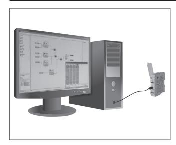
The CERTUS Configuration Software (CCS) is a userfriendly configuration tool to program the CMM in just a few simple steps. By clicking on the functional icons it is easy to "Drag&Drop" configurable safety functions.
