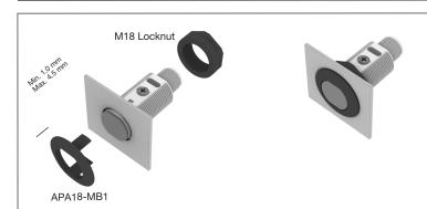
PA18 mounting with a combination of 1 x APA18-MB1 and 1 x M18 locknut.
