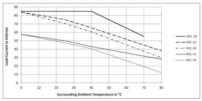
RGC...P models max. operating temperature is +  $70^{\circ}$ C / +  $158^{\circ}$ F
