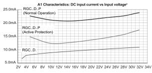
x:Input currents for RGC1..D15, RGC1..D20, RGC1..D25, RGC1..D30, RGC1..D4x, RGC1..D6x
