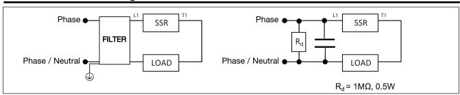
Note: The suggested filtering is determined by tests carried out on a representative setup and load. The RGC1P. is intended to be integrated within a system where conditions may differentiate from conditions utilised for tests, such as load, cable lengths and other auxiliary components that may exist within the end system. It shall be the responsibility of the system integrator to ensure that the sytsem containing the above component complies with the applicable rules and regulations.
