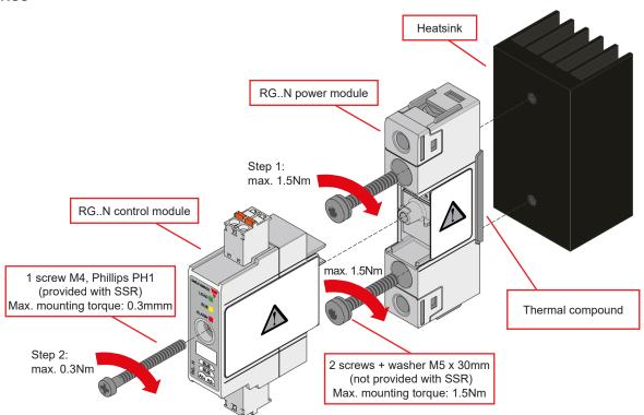
Step 1: Mount RG..N power module to Heatsink
