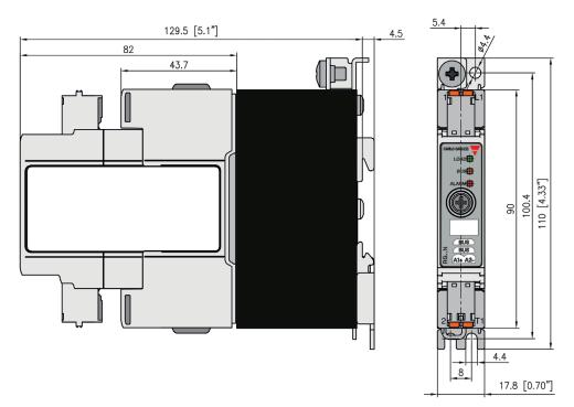
Housing width tolerance +0.5mm, -0mm as per DIN 43880. All other tolerances +/- 0.5mm. Dimensions in mm.
