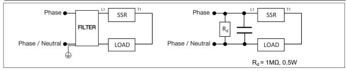
Note: The suggested filtering is determined by tests carried out on a representative setup and load. The RGS1P. is intended to be integrated within a system where conditions may differentiate from conditions utilised for tests, such as load, cable lengths and other auxiliary components that may exist within the end system. It shall be the responsibility of the system integrator to ensure that the system containing the above component complies with the applicable rules and regulations.
