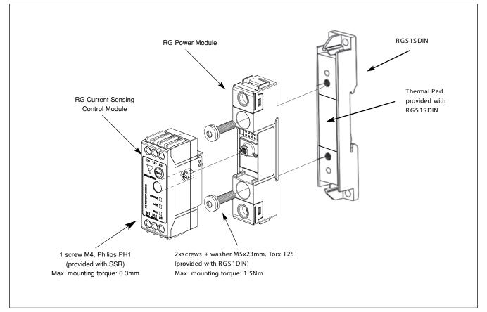
The RG Power Module is gradually tightened (alternating between the 2 screws) to a maximum torque of 1.5Nm.
