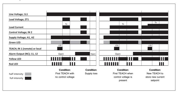
The TEACH procedure can be performed either locally or remotely. For local TEACH, the front 'TEACH' button on the SSR has to be pressed for at least 3 seconds (but less than 5 seconds). Remote TEACH can be performed by applying a high signal on terminal IN 1 for a duration of at least 3 seconds (but less than 5 seconds).
