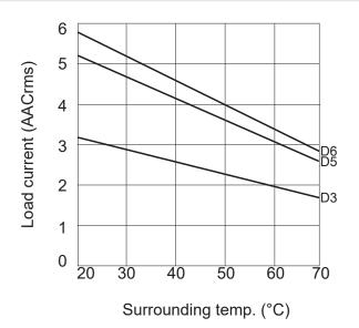
Derating curve is used for finding max. load current at an elevated ambient temperature. The 3 lines in the graph represent the 3 nominal current ratings of the RP1 series (RP1...D3/D5/D6).
