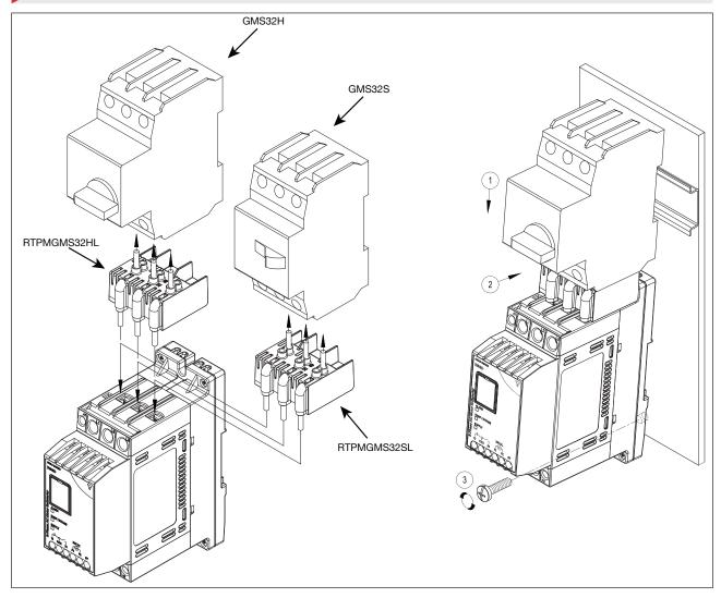
The following procedure should be followed when mounting the GMS motor starter onto the RSBD 45mm soft starter:-
