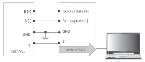
**Note:** To minimize the reflections from the end of the RS485 cable it is required to place a line termination near each of the 2 ends of the bus by a proper resistor.
