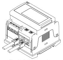
Fig. 18 RJ11 connections
