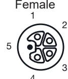
A circular diagram of a female M12 connector showing five pins labeled 1 through 5. Pin 1 is at the top, followed by 2, 5, 3, and 4 at the bottom. |
