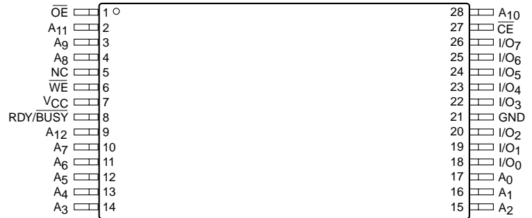
TSOP Package (8mm x 13.4mm) (H13)
