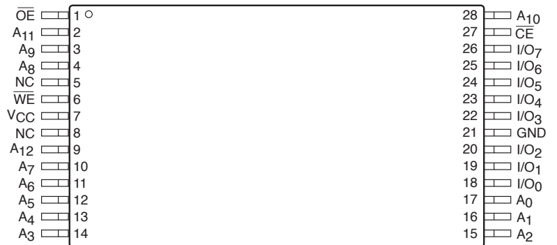
TSOP Top View (8mm x 13.4mm) (T13, H13)
