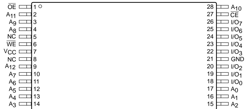
TSOP Top View (8mm x 13.4mm) (H13)
