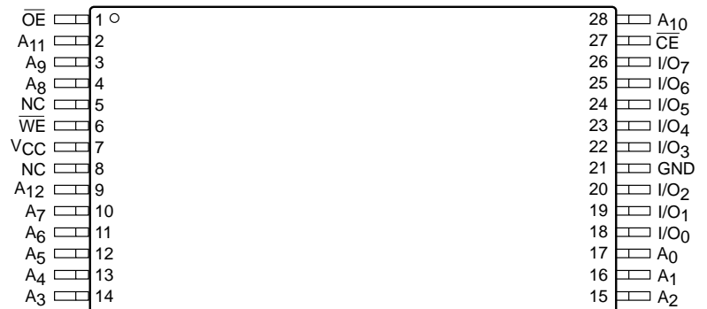
TSOP Top View (8mm x 13.4mm) (H13)
