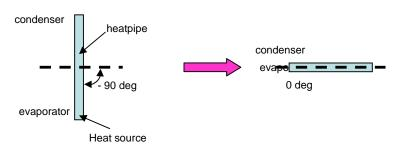
• The heatpipe performance is without change from -90 deg to 0 deg. Larger than 0 deg (i.e. evaporator is higher than condenser), the performance of grooved pipe will degrade 50%.
