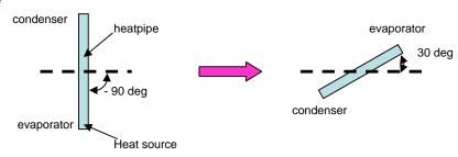
• Larger than 30 deg, the performance of mesh pipe will degrade 50%.
