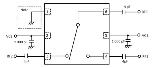
Note: It is recommended to connect the pin directly to the ground, or not to connect the pin to anything.
