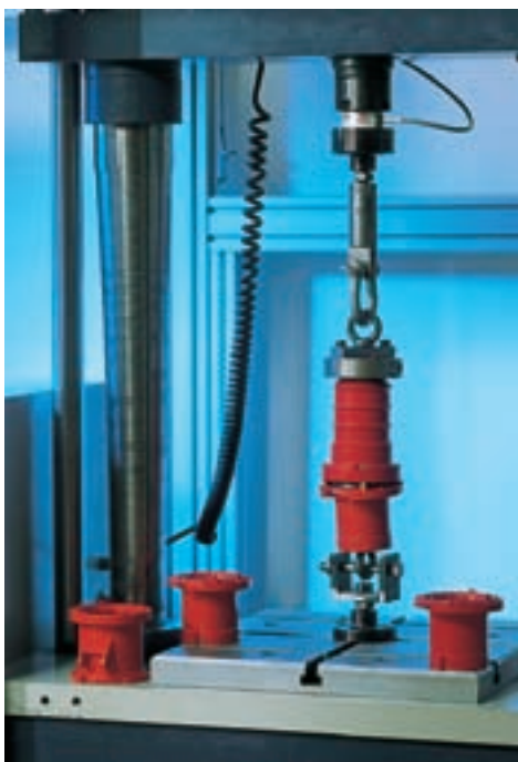
All injection moulded parts are subjected to tensile strength and pressure tests
