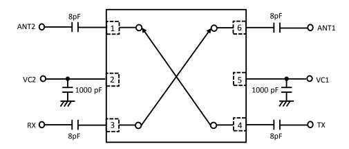
The application circuits and their parameters are for reference only and are not intended for use in actual designs. DC Blocking Capacitors are required at all RF ports.
