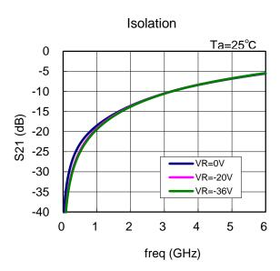
\*) Series configuration. Zo= $50\Omega$  . Losses of test fixtures are excluded from the measuring data.
