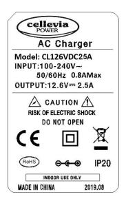
**Attention.** The charger is designed to work with a lithium-ion battery pack with a built-in balancer system. Its use for charging packages without a balancing system is only possible if the cell manufacturer allows such a possibility, e.g. for cells of the same type and from the same batch, and for charging with low current. If in doubt, please check the cell manufacturer's recommendations (datasheet) and follow the recommendations contained therein.
