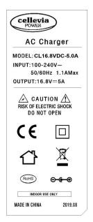
**Attention.** The charger is designed to work with a lithium-ion battery pack with a built-in balancer system. Its use for charging packages without a balancing system is only possible if the cell manufacturer allows such a possibility, e.g. for cells of the same type and from the same batch, and for charging with low current. If in doubt, please check the cell manufacturer's recommendations (datasheet) and follow the recommendations contained therein.
