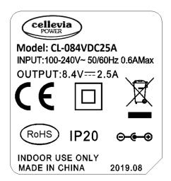
Attention. The charger is designed to work with a lithium-ion battery pack with a built-in balancer system. Its use for charging packages without a balancing system is only possible if the cell manufacturer allows such a possibility, e.g. for cells of the same type and from the same batch, and for charging with low current. If in doubt, please check the cell manufacturer's recommendations (datasheet) and follow the recommendations contained therein.
