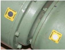
Two Jumbo-CelsiDot® 93°C temperature labels are applied to an electric motor and gear box. The motor housing passed the 93 °C level. The gear box never reached the 93 °C. The large white / black change area can easily be spotted from a remote location. Excellent for visual remote supervision
