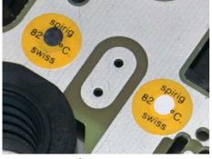
The CelsiPoint<sup>®</sup> shown here do cover only one specific temperature level (select from 40 different levels between 40 to 260 °C).On the left side the surface did exceed the 82°C level, on the right side not.
