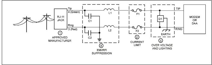
Figure 3. Telephone Line Interface.
