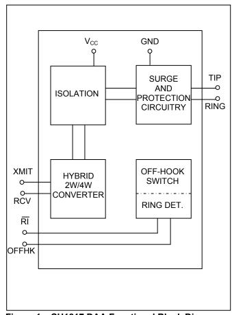
Figure 1. CH1817 DAA Functional Block Diagram.
