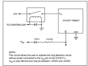
Figure 4. Low Power Ring Detection.
