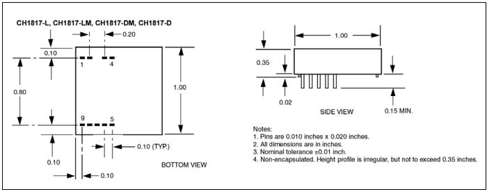
Figure 7. Mechanical Specifications.
