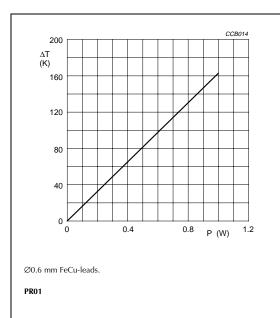
Fig.20 Hot-spot temperature rise ( $\Delta T$ ) as a function of dissipated power.
