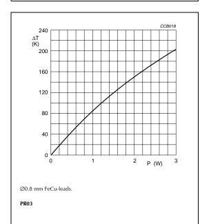
Fig.32 Hot-spot temperature rise ( $\Delta T$ ) as a function of dissipated power.
