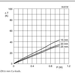
Minimum distance from resistor body to PCB = 1 mm.
