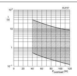
The graph is based on measured data under constant voltage conditions; these data may deviate according to the application.
