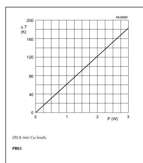
Fig.28 Hot-spot temperature rise ( $\Delta T$ ) as a function of dissipated power.
