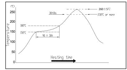
Temperature profile for reflow soldering
