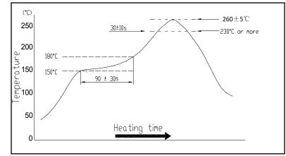
Temperature profile for reflow soldering
