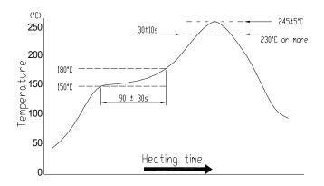
Temperature profile for reflow soldering
