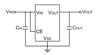
For CJ75XXS series, input and output capacitors are required to achieve stability and help the equipment obtain better transient response and PSRR. It is recommended to use  $1\mu F$  input and  $1\mu F$  output capacitors.
