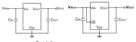
$C_{\text{IN}}$  :1.0 $\mu F$  or more  $C_{\text{OUT}}$  :1.0 $\mu F$  or more, 10 $\mu F$  is recommended
