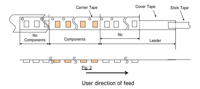
(4) Gap between Carrier Tape and Cover Tape Cover Tape protrudes from Carrier Tape by 0.5mm max.
