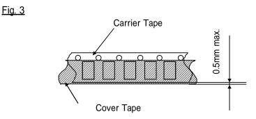
Holes of Carrier Tape are covered with Cover Tape by 0.75mm max.
